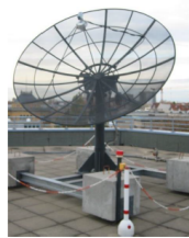
S-Band Antenna of TU Berlin (Ø 3m)
